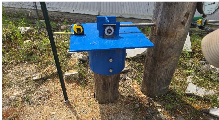
Figure 1: Pile Connection Test Setup
